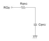
Reset gate clock equivalent circuit
