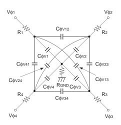
Vertical transfer clock equivalent circuit
