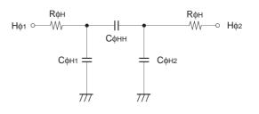
Horizontal transfer clock equivalent circuit
